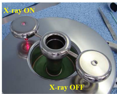
Figure 2: Picture showing the two "satellites" holding the CNT photocathodes. The backside of the upper left photocathode is illuminated.
