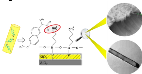
Figure 1. Scheme of drug loading in inner surface of silica nanotubes.
