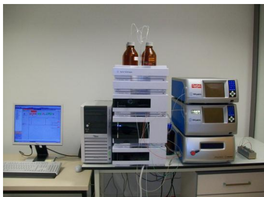
Figure 1. Set-up for a complete FFF-MALS system (Eclipse, DAWN, Optilab, Agilent HPLC)
