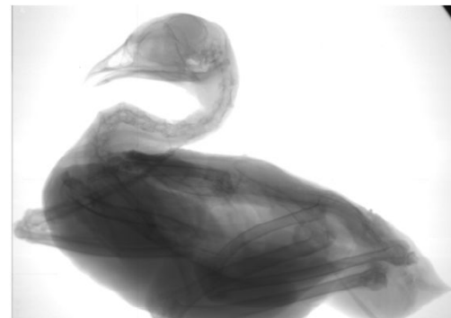
Figure 6: Image of a bird realised with a single CNT source.
